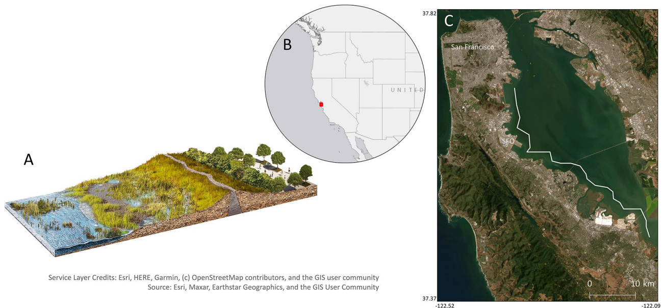
Fig. 1. Depiction of a horizontal levee (A) and study location (B and C). Transects used in the hydrodynamic simulations are shown by the white lines in (C). Maps in B and C created with ArcMap 10.7.1 ( https://desktop.arcgis.com/en/quick-start-guides/10.7/arcgis-desktop-quick-start-guide.htm ).
